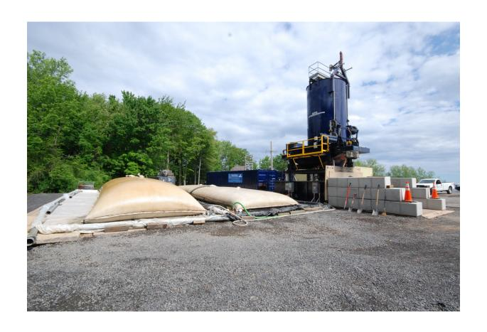
Primary Screening -Washing and Separation of Zebra Mussels From Silt-Clay and Held For 30 Days Prior Disposal or Reuse.
